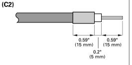
Fig. D RG8 Cable - Rear Exit
